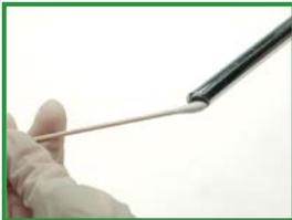
Cleaning the lens of an endoscope
