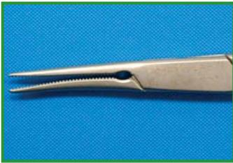
Deformation caused by improper handling
