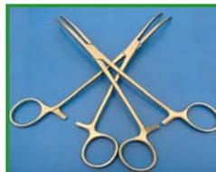
Contact corrosion between two instruments both made of stainless steel
