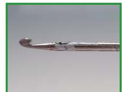
Standard chrome plate handcraft crochet hook – Chrome plate is not able to withstand reprocessing.
