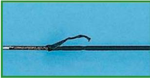
Damaged insulation on HF instrument
