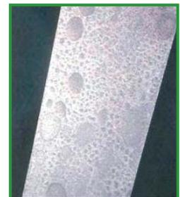
Instrument surface with drip-like discoloration
